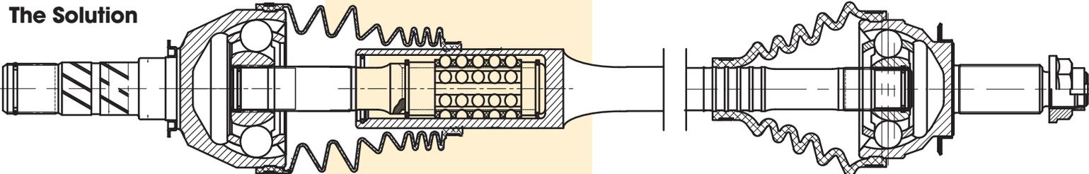
Developed for increased linear travel and greater articulation, to compensate for worn or fatigued engine / transmission mounts.
