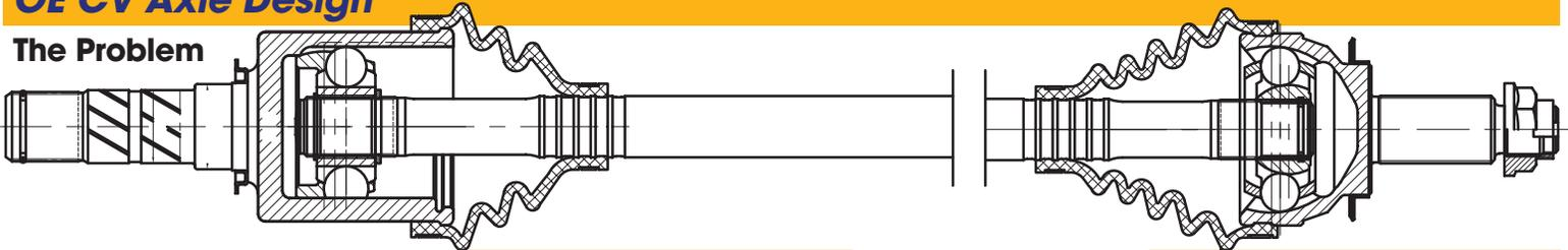
Developed from Original Equipment design. These CV axles rely on the inboard joint to provide all linear travel (plunge) for the CV axle.
